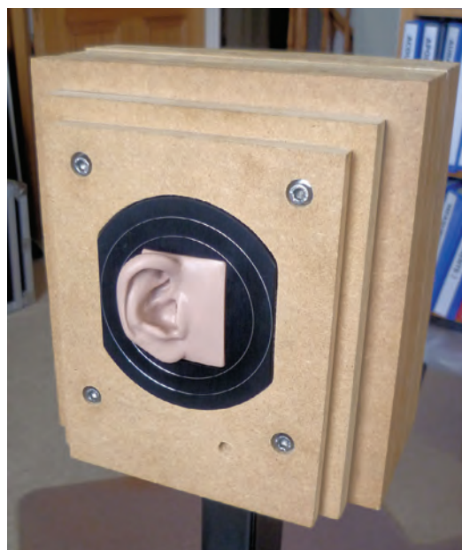
Figure 3. The artificial head used by the author for measuring headphones, which incorporates key elements of the GRAS 43AG ear and cheek simulator. Left and right artificial pinnae are used as appropriate
